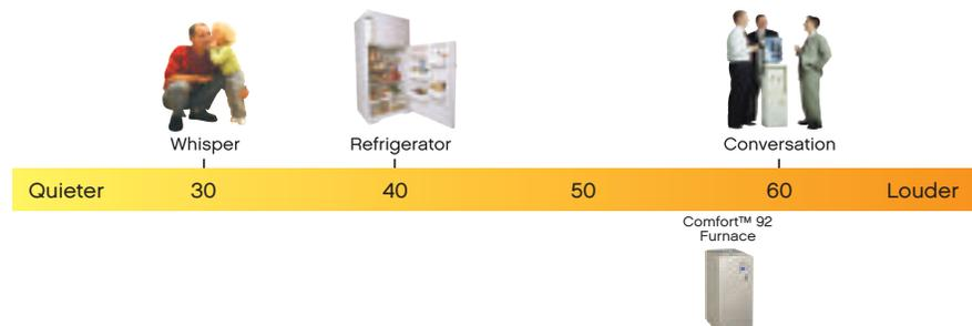
Carrier manufactures gas furnaces that are among the quietest in the industry. We test our products in a sound laboratory specifically built to resemble a typical residence. Sound level recordings produced at steady state, low fire operation (the most common operating condition), measured 3 feet from furnace. Other sound levels, mentioned for comparison, as published at <http://www.nidcd.nih.gov/health/hearing/ruler.asp>.
